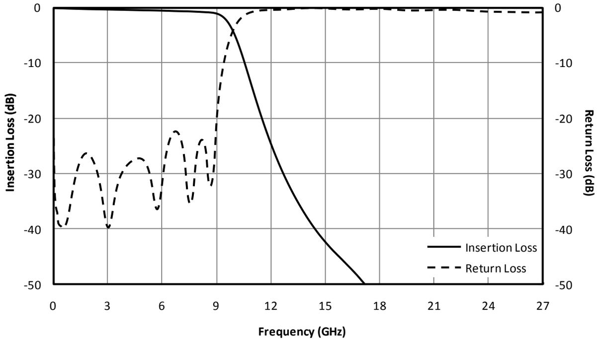
Fig. 1. Magnitude response for a typical FLP-0960.
