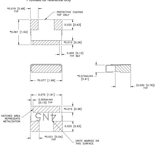
Unless Otherwise Specified: TOLERANCE: X.XXX = ± 0.005 DIMENSIONS APPLY BEFORE SOLDER ALLOW 0.015 MAX FOR PRETINNED SURFACES
