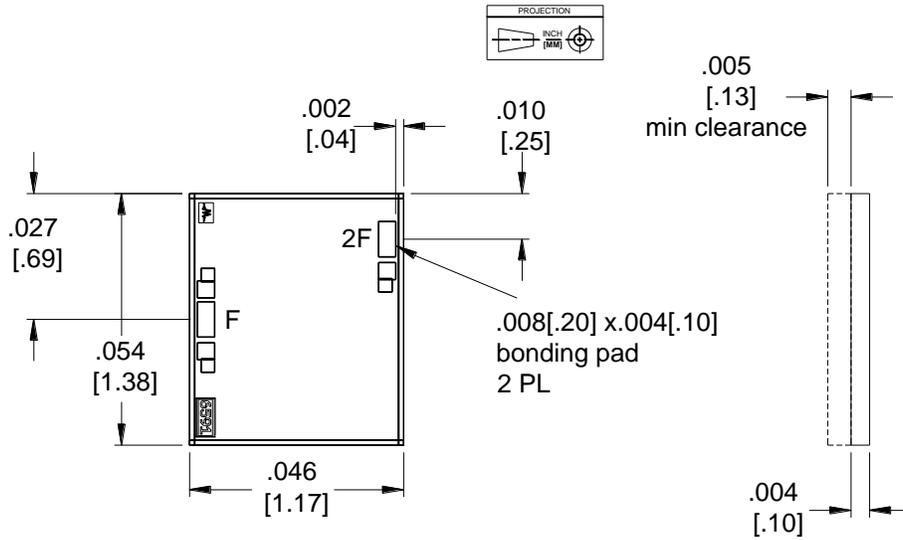
1. CH Substrate material is 0.004 in thick GaAs.
