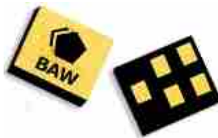
CSP-5CT package: 1.4 x 1.2 x 0.46 mm
