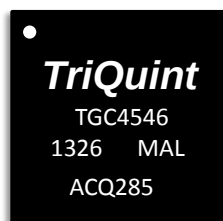
28-pin 5x5mm QFN package
