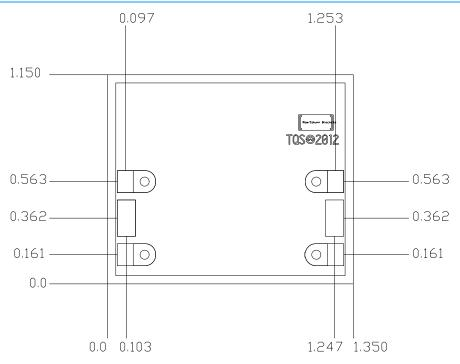
Unit: millimeters Thickness: 0.10
