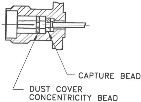
HOUSING: STEEL, CRES ALLOY UNS-S30300 PER ASTM-A582. PASSIVATE PER QQ-P-35.
