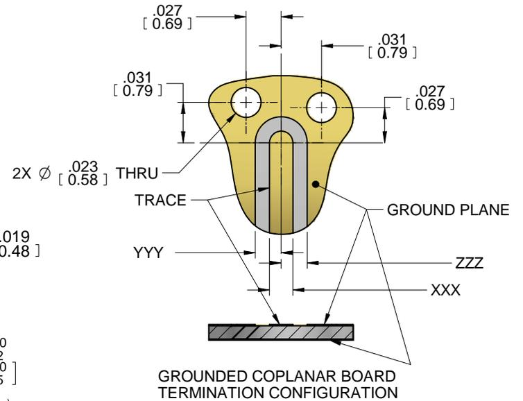
4. GROUND PLANE AND TRACE SPECIFIC CONFIGURATIONS TO BE DETERMINED BY INDIVIDUAL APPLICATION REQUIREMENTS.
