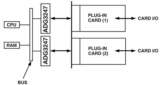
Figure 12. ADG3247 in a Hot Plug Application
