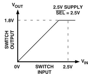
Figure 8. 2.5 V to 1.8 V Voltage Translation,  $\overline{SEL} = V_{CC}$
