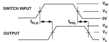
Figure 2. Propagation Delay
