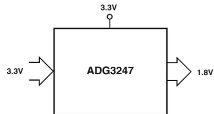
Figure 9. 3.3 V to 1.8 V Voltage Translation,  $\overline{SEL} = 0 V$
