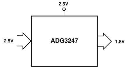
Figure 7. 2.5 V to 1.8 V Voltage Translation,  $\overline{SEL} = V_{CC}$
