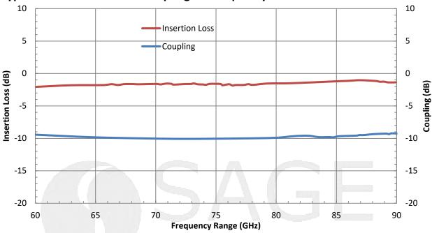
\*Insertion loss includes circuit loss
